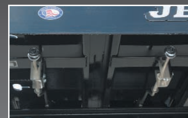
Dual remote winch releases mounted under deck for convenient operation of low-profile winches on lower deck.
